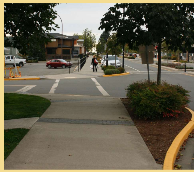
Curb extensions at block ends to slow vehicle turning speeds and provide opportunities for trees and landscape (Brentwood Bay, BC)
