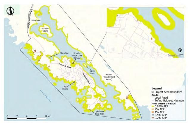
Figure 24: Comparison of the different AEP flood extents with 0 m RSLR at Ucluelet. Base layer: CARTO's Positron, created using derivatives of OpenStreetMap data - openstreetmap.org (© OpenStreetMap contributors; cartography license CC BY-SA).
