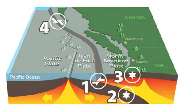
Figure 13: British Columbia earthquake hazard sources. See above text for description of the 4 earthquake sources (figure from Province of British Columbia, 2018).
