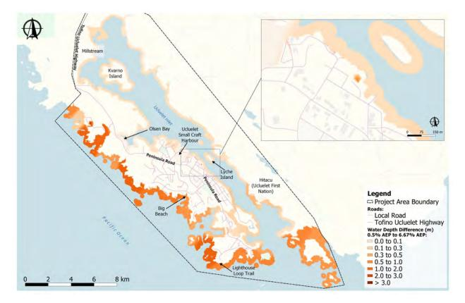
Figure 23: Coastal storm flood depth difference map between the rare (0.5% AEP) and frequent (6.67% AEP) floods for the future (1 m RSLR) scenario.
