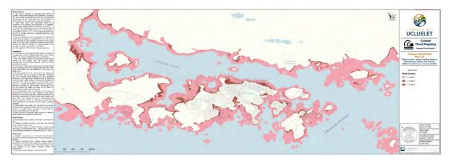
Figure 32: Maximum total water extents for the splay faulting rupture (Gao2018-S-A) with RSLR 0 m, 1 m, and 2 m. Total water depth includes maximum tsunami wave amplitude, earthquake subsidence, and high tide (HHWLT). This figure is intended to provide a snapshot of the full-scale maps found in the Map Atlas.
