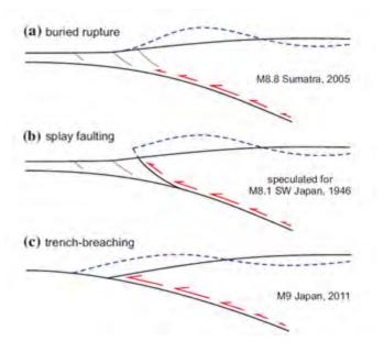
Figure 20: Megathrust earthquake rupture types and seabed deformation (dashed purple line) (Adapted from Wang and Tréhu, 2016).
