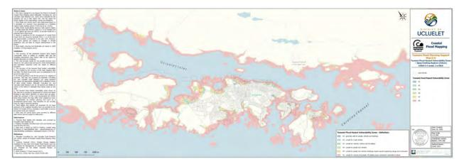
Figure 37: Tsunami flood hazard vulnerability zones for the DOU, based on the worst-case tsunami with 1 m RSLR.
