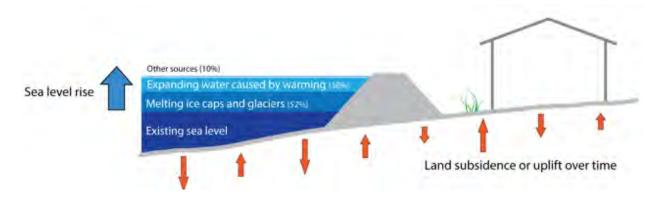
Figure 3: Drivers of RSLR including components of SLR and land subsidence or uplift—estimates of factors contributing to SLR are based on Union of Concerned Scientists (2015).
