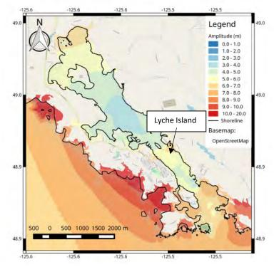
Figure 29: Maximum tsunami amplitude for splay faulting rupture (Gao2018-S-A) in metres relative to ambient water level. Ambient water level = 2 m tide (HHTWL) + 0 m RSLR (figure from Cascadia Coast Research Ltd., see also Appendix A).
