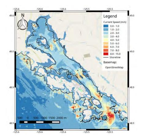
Figure 30: Maximum tsunami current speeds for splay faulting rupture (Gao2018-S-A) in metres per second. Ambient water level = 2 m tide (HHTWL) + 0 m RSLR (figure from Cascadia Coast Research Ltd., see also Appendix A).
