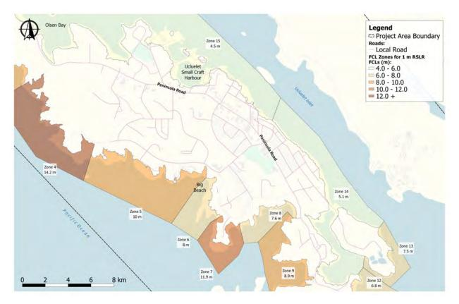
Figure 1: FCL reaches for an example area of the DOU, for the 1 m RSLR scenario.
