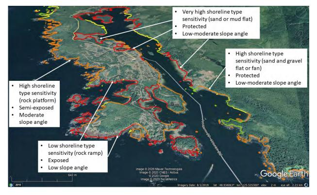
Figure 14: Shoreline sensitivity to sea level rise (Biffard and Stevens, 2014). Red indicates very high shoreline erosion sensitivity, orange indicates high sensitivity, yellow is moderate sensitivity, light green is low sensitivity and dark green is very low sensitivity. Annotations by Ebbwater.
