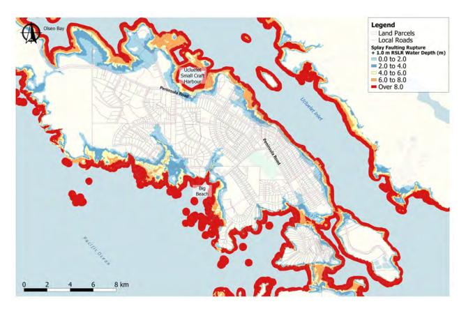
Figure 2: Tsunami flood depths for an example area of the DOU, for a tsunami generated by a splay faulting rupture, for the 1 m RSLR scenario.
