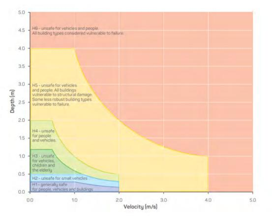
Figure 36: Combined flood depth and velocity curves (flood hazard curves) (AIDR, 2017).
