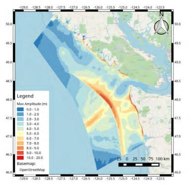
Figure 28: Maximum tsunami amplitude for splay faulting rupture (Gao2018-S-A) in metres relative to ambient water level. Ambient water level = 2 m tide (HHTWL) + 0 m RSLR (figure from Cascadia Coast Research Ltd., see also Appendix A).
