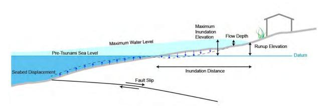
Figure 2: Features of a tsunami caused by an earthquake. The fault slip causes seabed displacement that generates the tsunami. Maximum water levels increase towards the shore due to shoaling (figure adapted from UNISDR, 2017).
