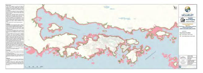
Figure 33: Maximum total water extents for the two rupture models with RSLR 0 m. Total water depth includes maximum tsunami wave amplitude, subsidence due to the earthquake, high tide (HHWLT), and RSLR. This figure is intended to provide a snapshot of the full-scale maps found in the Map Atlas.
