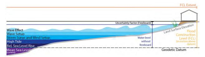
Figure 5: Conceptual drawing of the Flood Construction Level (FCL).
