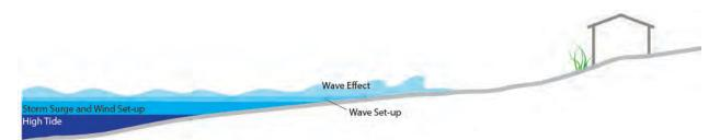
Figure 1: Components of total water level (total water level is composed of tide, storm surge, wind set-up, wave set-up and wave runup).
